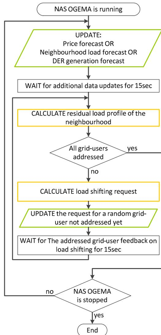
Figure 2 Flowchart of optimal load shifting planning application
